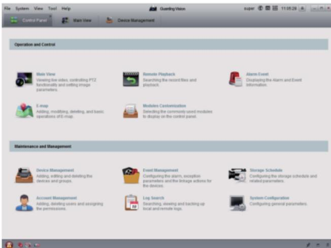
4. Go to **Control Panel-Device Management-Device**. At the bottom of the screen and in the **Online Devices** section, the screen will display all devices on the network. Create a password to activate the device if the device's status is inactive.
