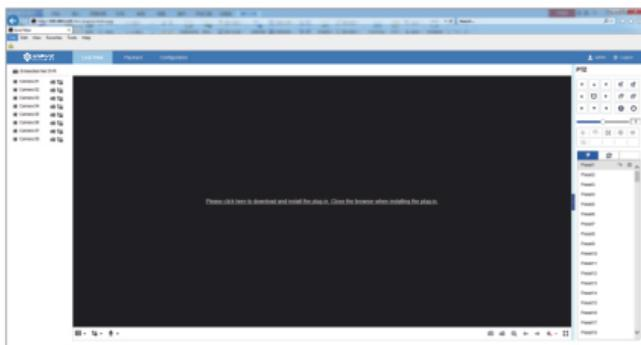
6. Re-open the IE browser and log in the camera. Choose the channel you want to access and set up the camera by clicking Configuration.
