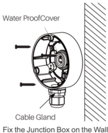
6. Route the cables through the cable hole. Here we take bottom cable hole as the example to describe the installation.
