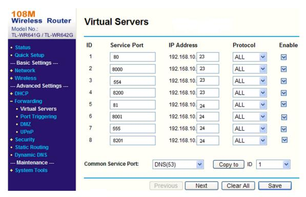
Figure 8-1 Port Mapping on Router
